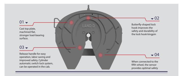
The LD-3510 plate and legs are made of cast steel with better tensile strength, which has excellent strength and durability. It can ensure the safe transportation of various large containers and other heavy equipment. This product has been used by Shacman and Sinotruk for more than ten years, and has won unanimous praise from customers for its convenience and speed.
